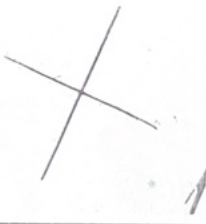
Two crosses overlaying one another, written in separate lithographic steps following realignment of the specimen. Placement accuracy is 2-3nm; the lines themselves are 16nm wide.
